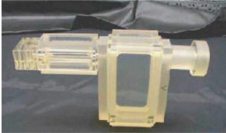
Figure 4.5: A picture of the Zerodur ultra-high vacuum cell.
