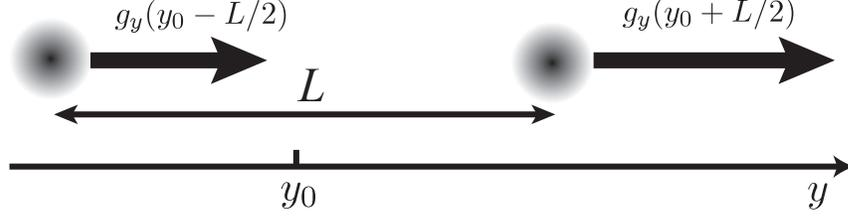
Figure 1.2: Gravity gradient measurement by differential accelerometers.
