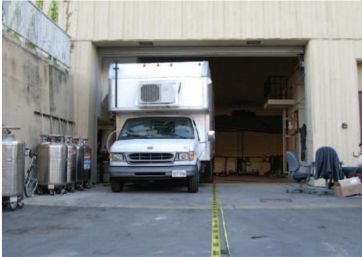
Figure 8.3: Truck during gravity gradient survey. Truck is driven by an electric motor to take measurements along a linear profile. Apparatus is about 2.1 meters above the ground.
